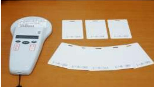
Figure 6. The RFID reader and tags
