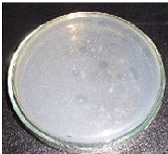
Fig. 3. The number of PHB/V degraders was estimated by the clear-zone technique
