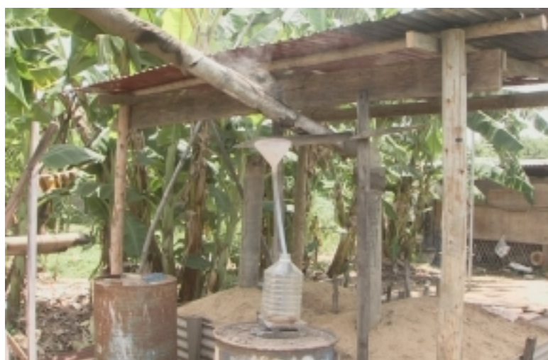
Fig. 2. (a) Put tile at the top of the chimney. (b) The steam is condensed into liquid. (c) Collect the vinegar drops from the bamboo or plastic pipe.
