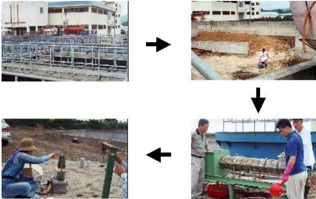
Fig. 1. Removing excess water from the starch sludge. (Clockwise, from top left); View of starch factory; Storage of sludge; Pilot screw press; Determining the water content by a far infrared moisture analyzer
