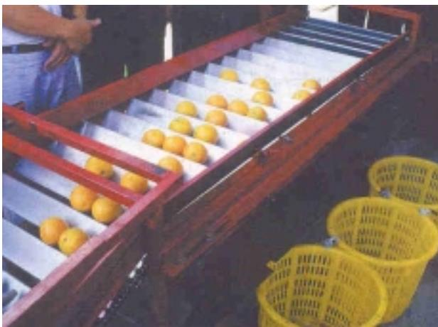
11-9. Mechanized grading of fruit by size, using slats
