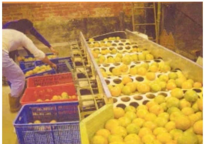
Fig. 11-7. (left) and Fig. 11-8. Mechanized grading of fruit by size, using different types of revolving drum
