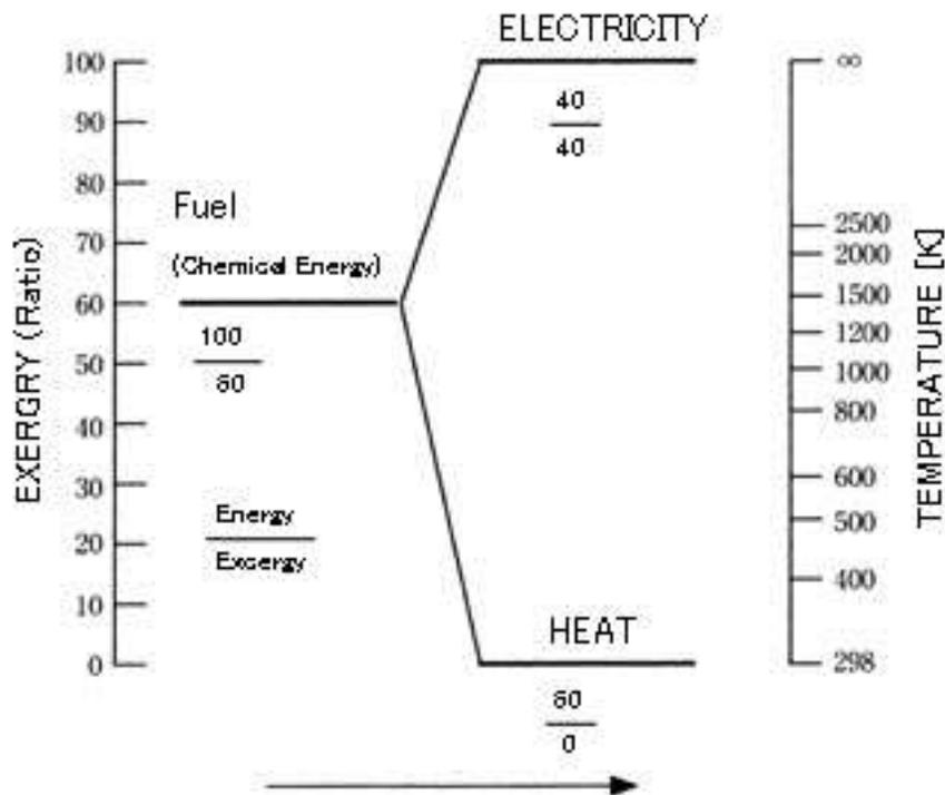
Fig. 2 Exergy/Energy Flow Electricity Generation (from Tsutsumi, Yoshida, 1999)
