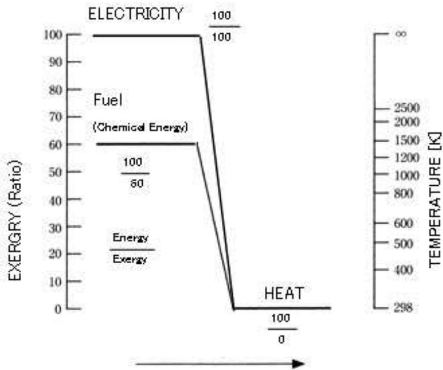
Fig. 3 Energy/Exergy Flow Direct Combustion
