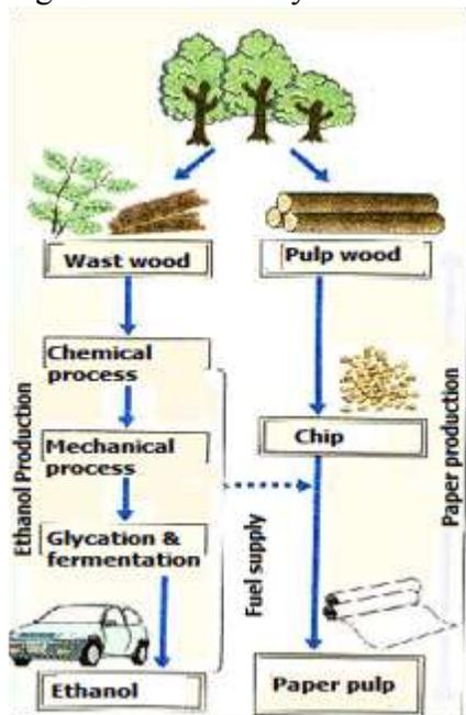
Fig. 16 Bioethanol from timber
