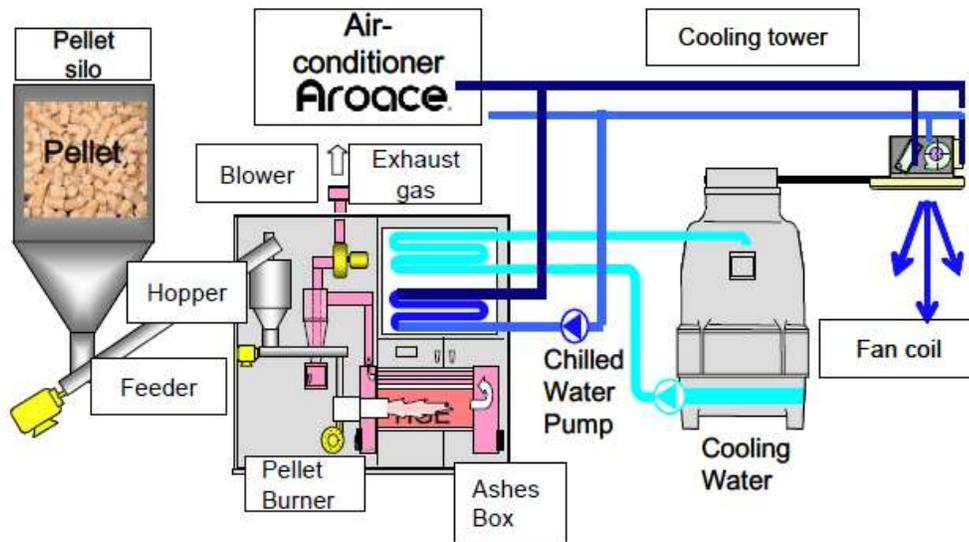
Figure 8. System of Pellet Fired Absorption Chiller-Heater
