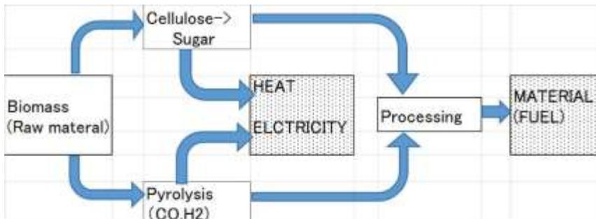
Fig.14 The Scheme of Bio-Refinery
