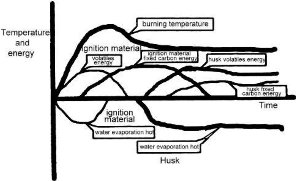
Fig.4. Energy change diagram in a furnace
