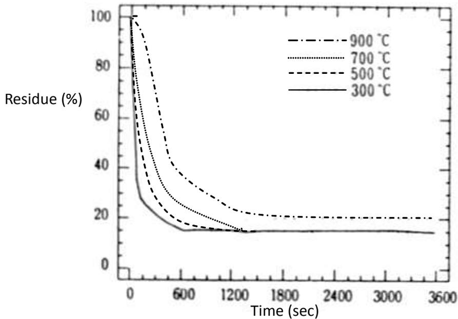
Fig. 1. The rice husk combustion curves with different temperature (moisture 12%) (Wong and Fon,1993).
