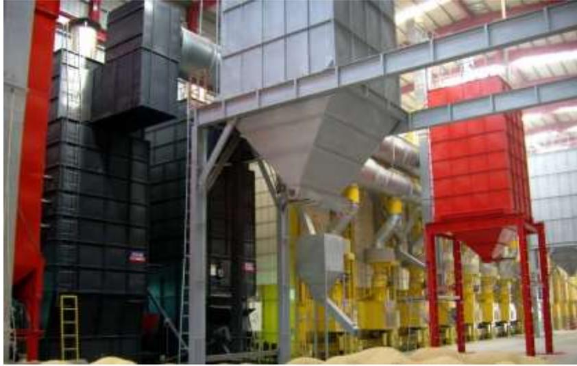
Fig. 5. The rice husk furnace with feeding facilities. (Suncue, 2014)
