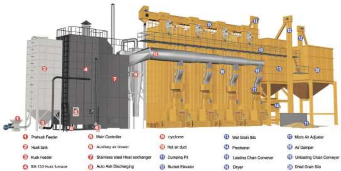
Fig. 11. A layout of a rice drying system with furnace (Suncue, 2014)
