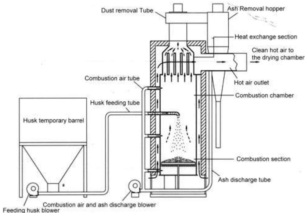
Fig. 9. A schematic diagram of rice husk furnace. (Suncue, 2014)
