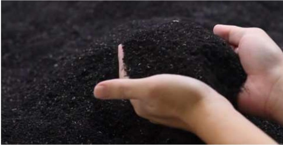
Fig. 2. Carbonized rice husk produced by a husk furnace
