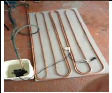
Fig. 2. Heat absorber design
